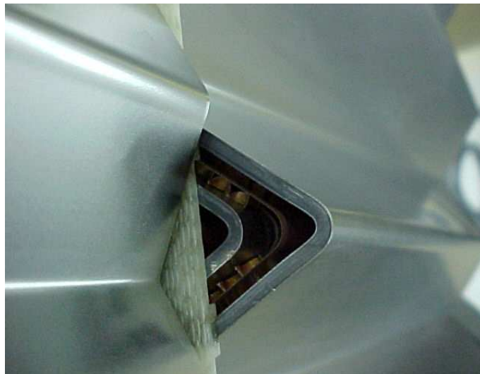
Figure 3.2: Stacked layer. The electrode is placed in between two absorbers.
