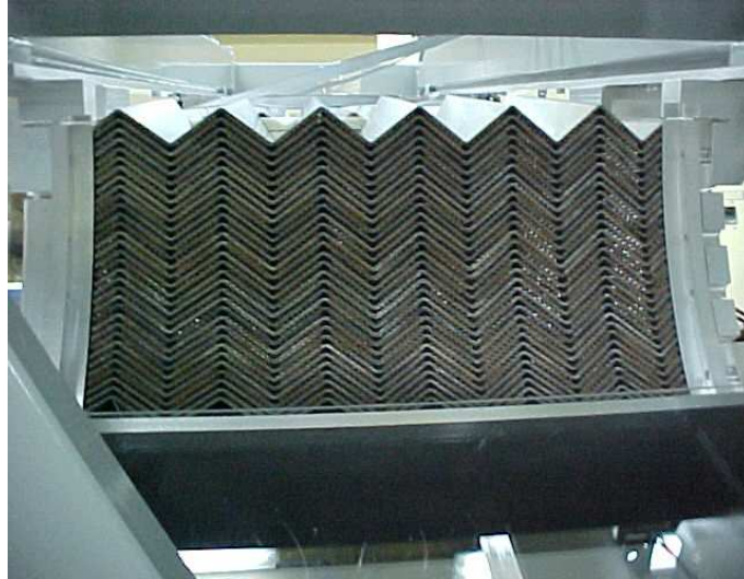
Figure 3.1: Accordion shape in EMEC inner wheel
