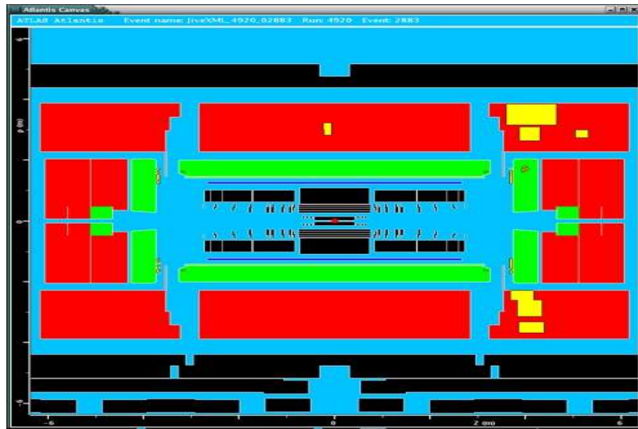
Figure 6.7: Cosmic muon event displayed using the Atlantis program crossing the EMEC-A wheel. The Hadronic Calorimeter is in red, while the Electromagnetic Calorimeter is in green. The muon cross from top to bottom depositing energy in both top and bottom EBA Tile towers and in the EMEC-A (small spot in grey).
