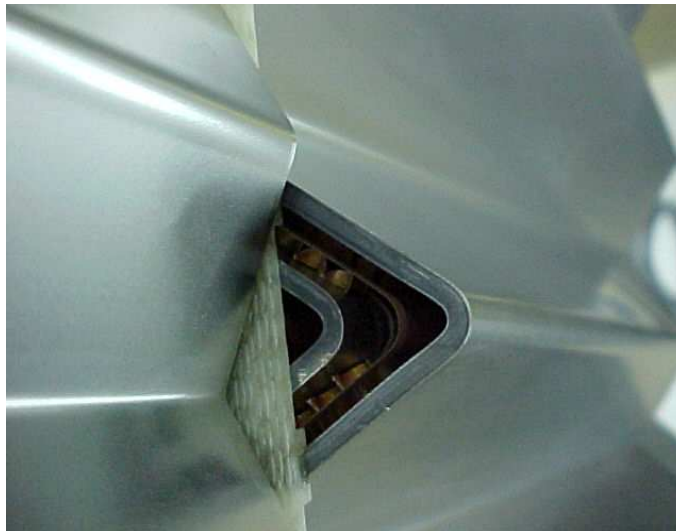
Figure 4.3: Stacked layer of the inner wheel. The electrode is placed in between two absorbers.
